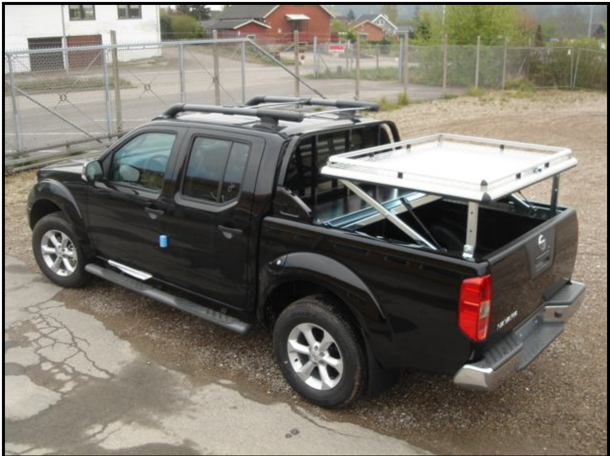
6 different positions allows to carry loads with various heights
